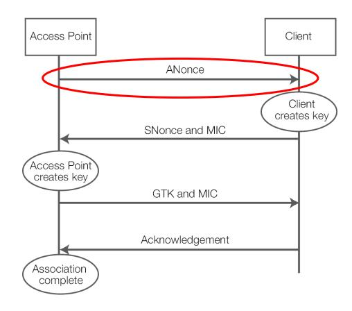
• The STA sends its own nonce-value (SNonce) to the AP together with a Message Integrity Code (MIC), including authentication, which is really a Message Authentication and Integrity Code (MAIC), and the Key Replay Counter which will be the same as Message 1, to allow AP to match the right Message 1.
