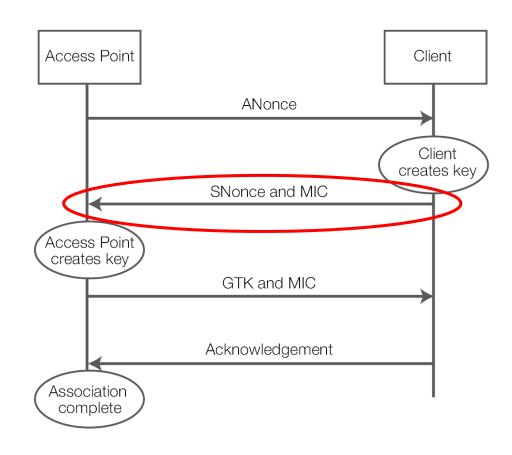
• The AP verifies Message 2, by checking MIC, RSN, ANonce and Key Replay Counter Field, and if valid constructs and sends the Group Temporal Key with another MIC.
