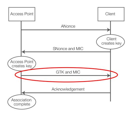
• The STA verifies Message 3, by checking MIC and Key Replay Counter Field, and if valid sends a confirmation to the AP.
