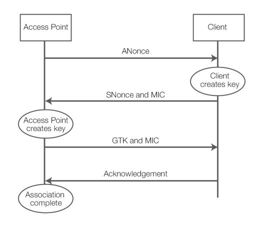
• The AP sends a nonce-value (ANonce) to the STA together with a Key Replay Counter, which is a number that is used to match each pair of messages sent, and discard replayed messages. The STA now has all the attributes to construct the Pairwise Transit Key (built with Preshared Key).
